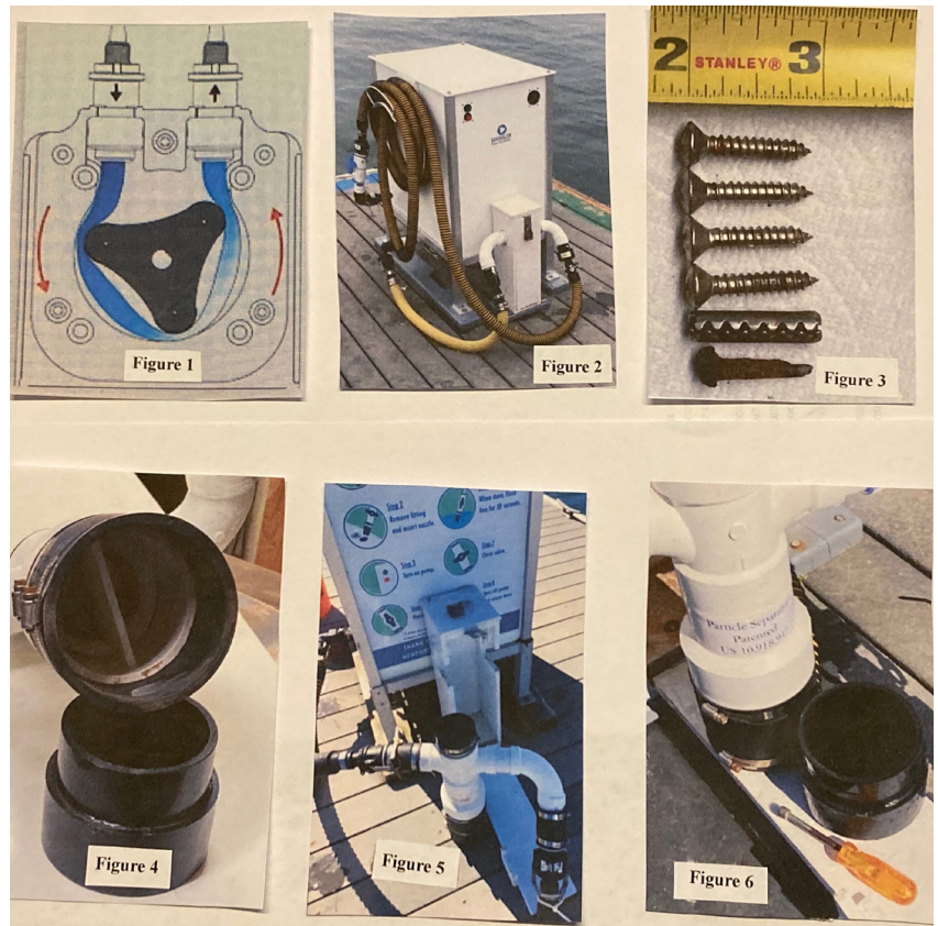
Figure 1: Internal hose of a peristaltic pump; Figure 2: Pumpout unit with locked wooden housing for the Particle Separator; Figure 3: Screws that have been caught by Particle Separator; Figure 4: Internal view of the Particle Separator; Figure 5: External view of the Particle Separator; Figure 6: Particle receiver. Photo: George Hylkema.
